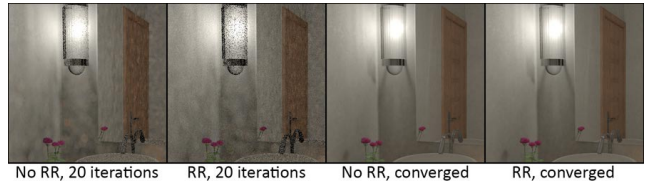
Fig. 5 Fragment reduction with Russian Roulette (RR) during splating, trading variance for a substantial decrease in both direct and indirect splating times.
