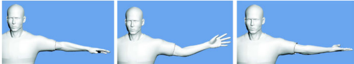
Figure 17. Avoidance of the typical LBS “candy-wrapper” artifact. (Left) is a reference pose, (middle) upper arm is rotated 90° about its axis, and on (right) upper arm is rotated 180° about its axis.
